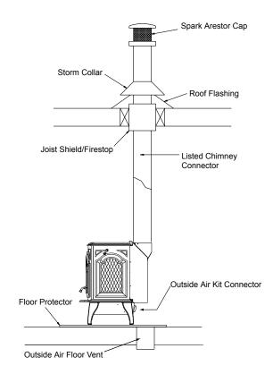
WARNING: NEVER DRAW COMBUSTION AIR FROM A WALL, FLOOR OR CEILING CAVITY OR FROM ANY ENCLOSED SPACE SUCH AS AN ATTIC OR GARAGE.
